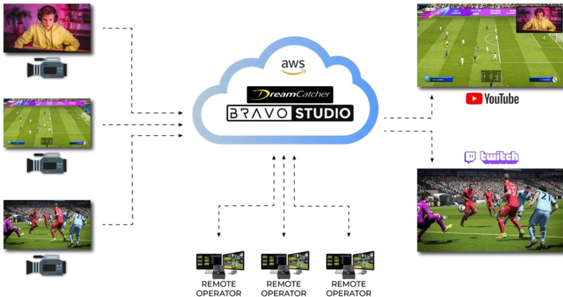
Using NDI, SRT, RIST, RTMPE and RTMPS protocols, multiple sources in different formats can be sent to a DreamCatcher™ BRAVO Studio in the cloud, where EA CGE operational staff can log in to access feeds, produce live shows, isolate replays, edit highlight packages, and send produced content to a Media Asset Management (MAM) service or distribution platform in the cloud for playout to content distributions networks (CDNs) – all from the comfort of their own homes.
